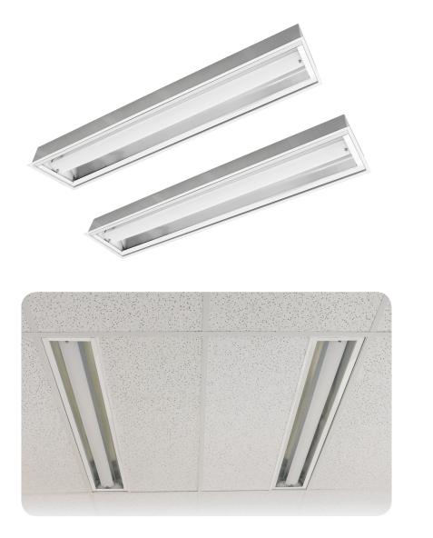
Installation: Surface Mount: Four .312" diameter holes. Grid Mount: Designed for 1" grid. Includes hardware to secure hanger wire. Flange Mount – Mounting yoke brackets (standard): Fixture mounting hardware included. Flange Mount – Install Frame (Accessory): Positively locates yoke brackets within ceiling opening; assures alignment of fixture. No measuring for yoke required; no drywall backing required (included with frame assembly).
