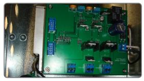
The power supply generates 12V from 100 – 240 VAC for each solenoid. There are three (3) connections (1 per solenoid) and two (2) connections (1 per each electric brake handle).
