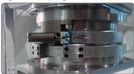
The springs generate friction by pulling the brake shoes towards the center drum, preventing the bearing from rotating freely.
